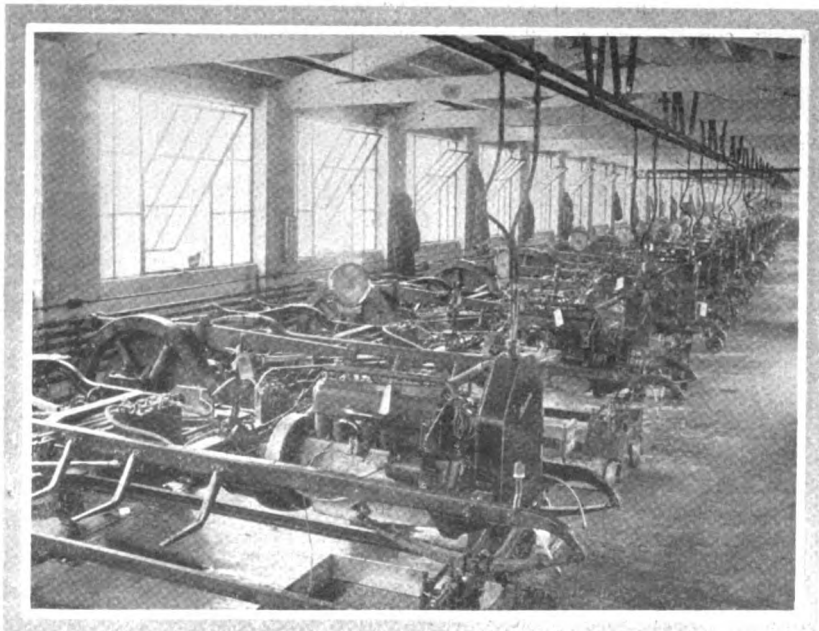
Studebaker chassis testing room showing six-cylinder cars undergoing their first trial under load. There is room for nineteen cars at one time in the 300-foot building. Each radiator connects to the circulating water mains which communicate with a tank. The gasoline is also supplied to each chassis from a main pipe
